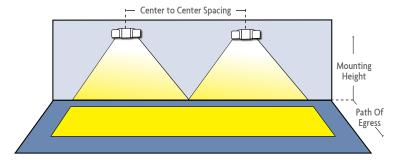
Compliant NFPA 101 requires 1.0 foot-candle average and 0.1 footcandle minimum with a 40:1 maximum/minimum ratio.
