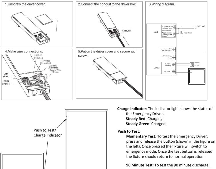
press and hold the button (shown in figure on left) for 5 seconds. The fixture should enter emergency mode for 90 minutes then return to normal operation. To exit at any time press and hold the test button for 5 seconds.
