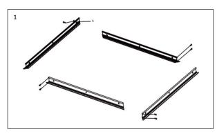
1. Remove accessories from the package carefully. Put together the four-piece drywall flange kit by using the supplied Wafer Head Self Tapping Screws . (Fig 1)
