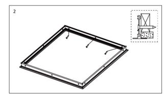
2. Place the assembled drywall flange kit into the corresponding hole and secure it to the hole with the countersunk head self tapping screws. (Fig 2)
