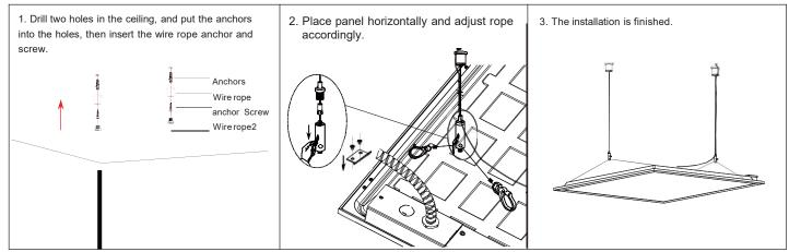
Note: 2\*2ft & 2\*4ft and 2\*2ft: 2 pcs suspension kits needed for installation. Emergency Fixtures: 3pcs suspension kit is needed for installation.
