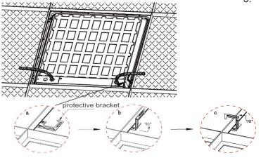
5. Grid clips are provided for additional retention to ceiling system. Orient the tabs on back of the fixture over the grid by bending tabs up 90 degrees perpendicular to back of the fixture. Next bend tabs 90 degrees towards T-GRID frame (Fig.3)
