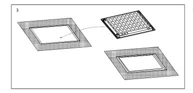
3. Place the panel into the flange kit and connect the input lines. Installation complete. (Fig 3)
