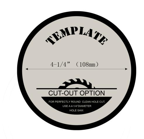
Cut out template and use it as your guide for cutting the fixture opening in sheetrock or other material. For best results, cut on the line to avoid making the opening too large.
