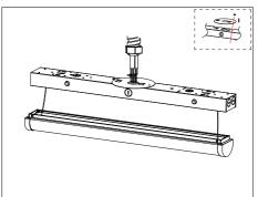
7. Locate the surface mounting holes and securely mount the housing directly to a sturdy surface using the correct mounting hardware. For reference, mounting holes are spaced 36 1/4" on 4' model and 83 3/8" apart on the 8' model.
