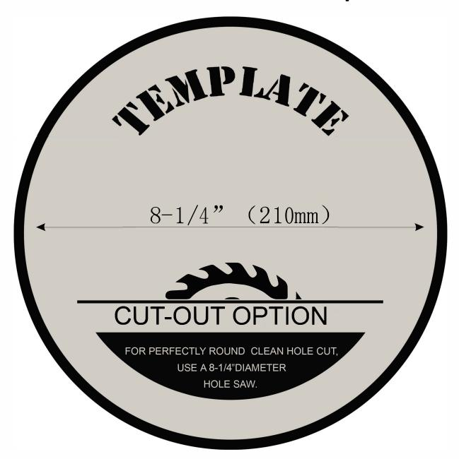
Cut out template and use it as your guide for cutting the fixture opening in sheetrock or other material. For best results, cut on the line to avoid making the opening too large.
