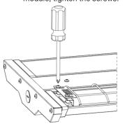
STEP 2 - Recess the metal plate into the fixture end cap, tighten
