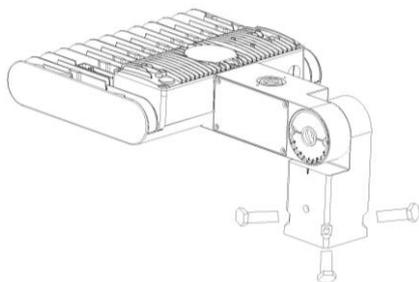
Adjust the fixture orientation by turning the bolt. In the above photo for the rocker installation hole, and for the sensor installation use the hole in the bottom.
