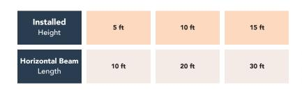
The length of the beam is about twice the size of the installed height.
